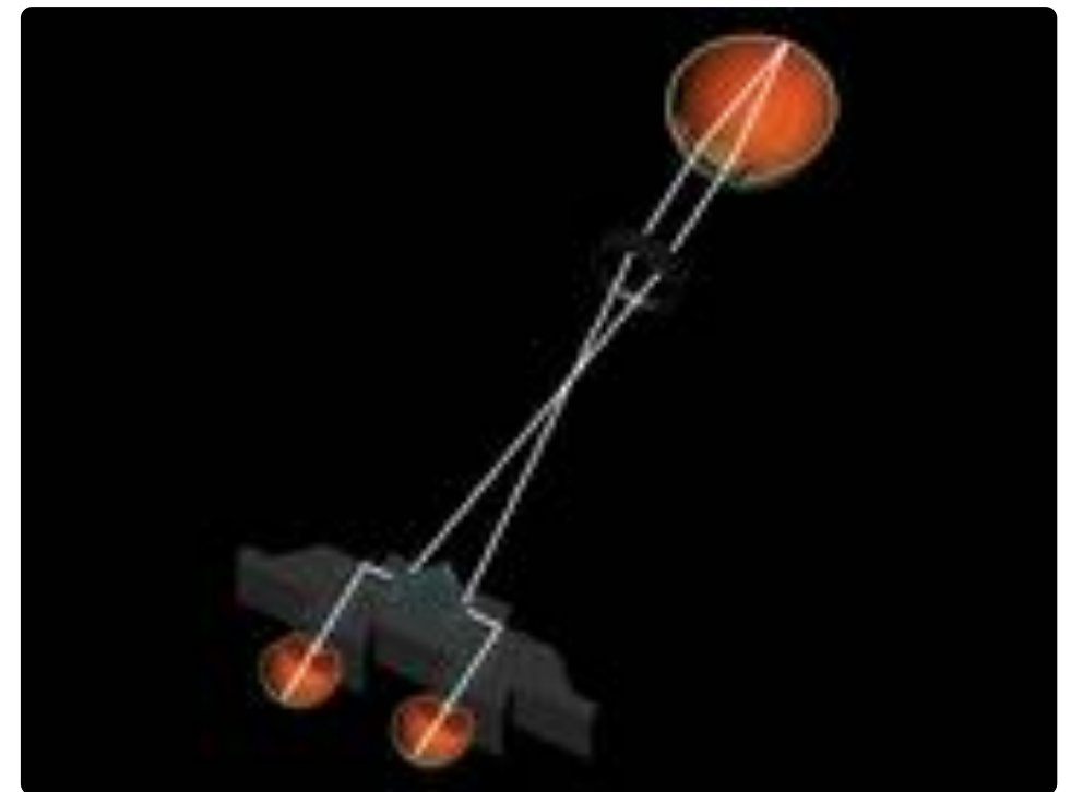
Figure 2.4 Simplified optics of the indirect ophthalmoscope
